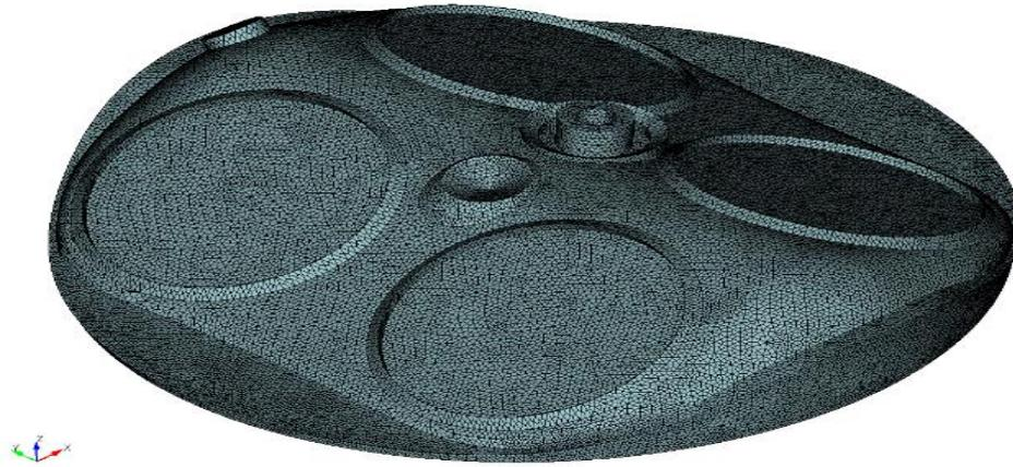
Figure 2: Spectral element skeleton of the fully-conforming hexahedral mesh of the cylinder head after the TET-to-HEX conversion.
