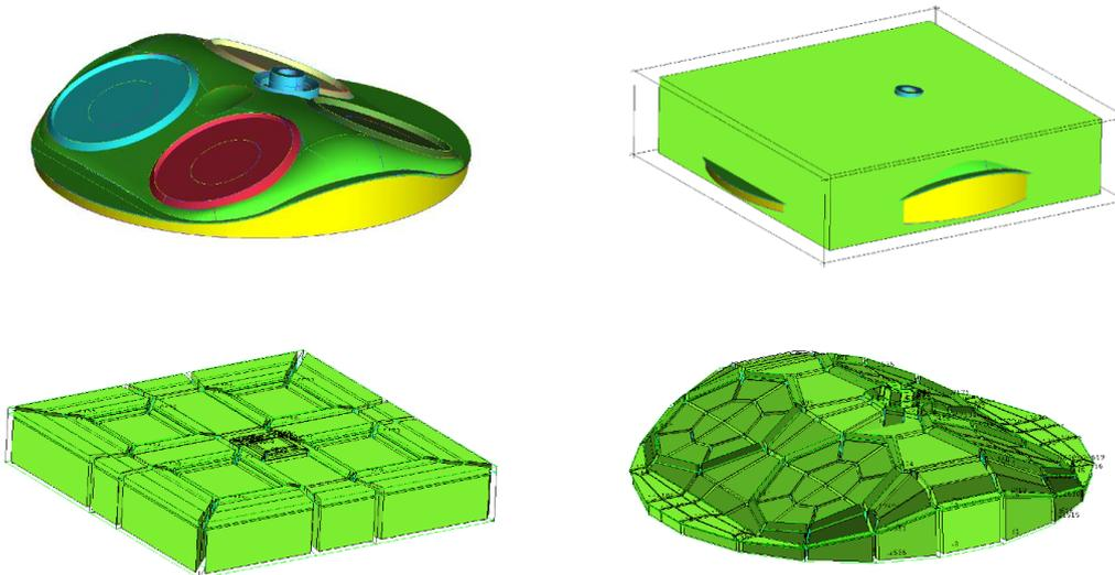
Figure 1: Block meshing using ICEM-CFD.
